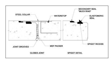
Figure 1 - J Series Jacking Pipe Joint
